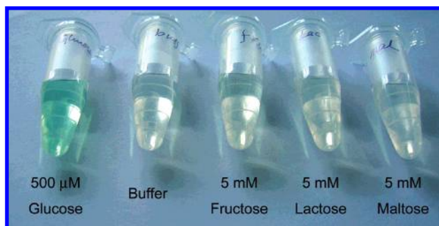
Figure 8. Typical photographs for glucose detection with the colorimetric method developed using GOx and the as-prepared \text{Fe}_3\text{O}_4 MNPs (from left to right: 500 \mu\text{M} glucose, buffer, 5 mM fructose, 5 mM lactose, and 5 mM maltose.).
