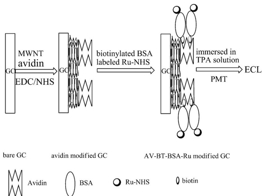
Scheme 1. The schematic diagram of ECL quantification of model BSA.
