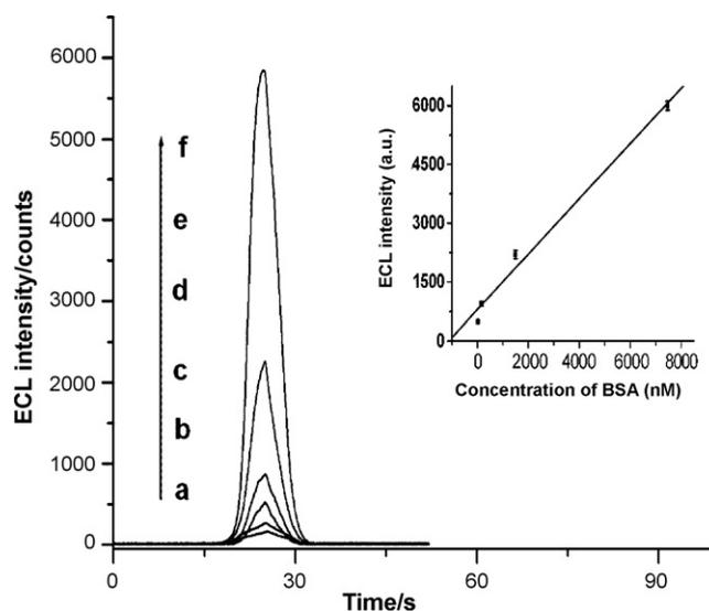
Fig. 3. ECL profiles of AV-BT-BSA-Ru-modified electrodes of different concentrations of BSA after immersed in a TPA-containing electrolyte solution. The concentrations of BSA are (a) 0, (b) 1.5 nM, (c) 15 nM, (d) 150 nM, (e) 1.5  $\mu$ M, and (f) 7.5  $\mu$ M. The inset is the linear relationship between the ECL intensity and the concentration of BSA. The conditions of ECL measurements are the same as in Fig. 2.
