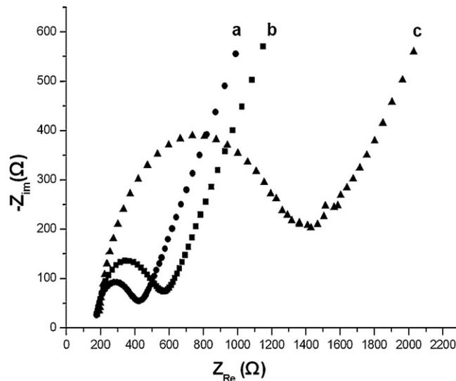
Fig. 1. Nyquist plot for the Faradaic impedance measurements in the buffer containing 1 mM  $\text{K}_3[\text{Fe}(\text{CN})_6]/\text{K}_4[\text{Fe}(\text{CN})_6]$  (1:1) as redox probe and 0.1 M KCl as supporting electrolyte. (a) A bare GC electrode, (b) an avidin-modified GC electrode, and (c) the avidin-modified electrode after incubation with 0.1 mM biotinylated BSA-Ru.
