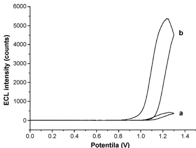
Fig. 2. ECL intensity vs. potential profile for the comparison of biotinylated BSA-Ru with non-biotinylated BSA-Ru attached to the avidin-modified electrodes under certain conditions. (a) Non-biotinylated BSA-Ru and (b) biotinylated BSA-Ru. The BSA concentration was 0.5 mM. ECL experiments were carried out in 50 mM TPA/0.1 M PBS electrolyte solutions at a scan rate of 50 mV/s. The sweep potential range is from 0 V to 1.3 V.
