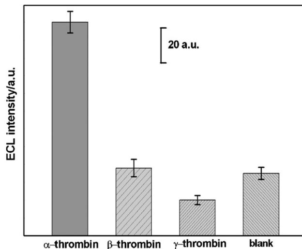
**Fig. 6** – Investigation of the specificity of the ECL aptasensor to the target  $\alpha$ -thrombin by comparing with  $\beta$ - and  $\gamma$ -thrombins as negative control and with the blank experiment. The concentration of  $\alpha$ -thrombin was 400 nM and the concentration of  $\beta$ - and  $\gamma$ -thrombins was  $\sim 800$  nM. The error bars indicate R.S.D.s of four replicate experiments.
