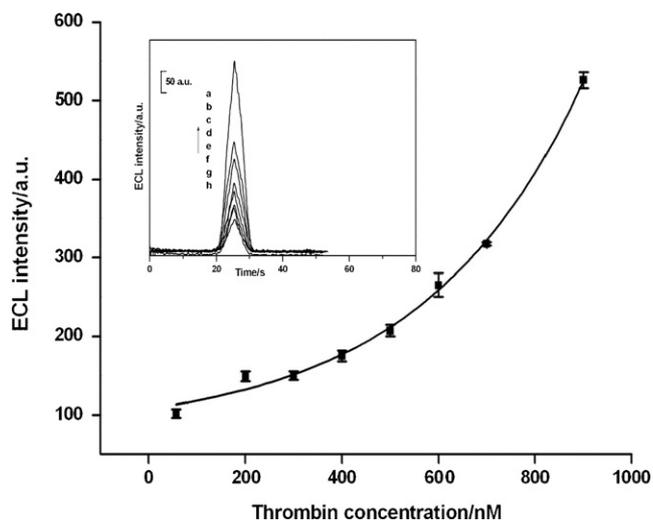
**Fig. 5** – Calibration curves of response-to-dose for thrombin with Sigmoidal (Boltzmann) regression. ECL responses for different concentrations of thrombin were given in the inset. (a) 56 nM, (b) 200 nM, (c) 300 nM, (d) 400 nM, (e) 500 nM, (f) 600 nM, (g) 700 nM, and (h) 900 nM. The error bars represent R.S.D.s of four replicate experiments.
