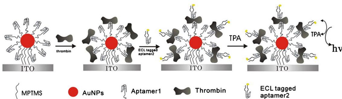
Fig. 1 – The schematic diagram of fabrication of ECL aptasensor.
