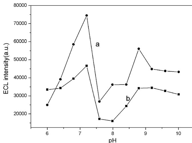
Fig. 4. Effect of buffer pH in the detection reservoir on ECL intensity: (a) ECL intensity of 10  $\mu\text{M}$  heroin, (b) ECL intensity of 10  $\mu\text{M}$  cocaine. Conditions: running buffer, 20 mM phosphate–acetate (pH 7.2); 5 mM  $\text{Ru}(\text{bpy})_3^{2+}$  with 50 mM phosphate–acetate buffer in the detection reservoir; detection potential, 1.2 V; electrokinetic injection, 6 s at 17 kV; separation voltage, 10 kV.
