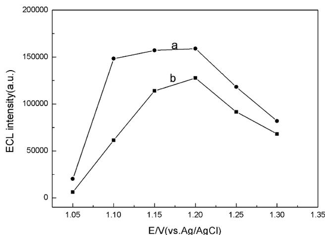
Fig. 2. Effect of detection potential on the ECL intensity: (a) ECL intensity of 10  $\mu\text{M}$  heroin, (b) ECL intensity of 10  $\mu\text{M}$  cocaine. Conditions: running buffer, 20 mM phosphate–acetate (pH 7.2); 5 mM  $\text{Ru}(\text{bpy})_3^{2+}$  with 50 mM phosphate–acetate buffer (pH 7.2) in the detection reservoir; electrokinetic injection, 6 s at 17 kV; separation voltage, 10 kV.
