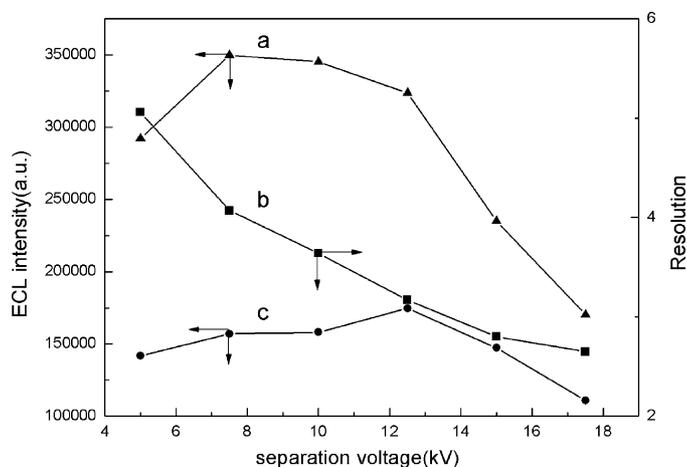
Fig. 3. Effect of separation voltage on ECL intensity and resolution: (a) ECL intensity of 10  $\mu\text{M}$  heroin, (b) resolution between heroin and cocaine, (c) ECL intensity of 10  $\mu\text{M}$  cocaine. Conditions: detection potential, 1.2 V; running buffer, 20 mM phosphate–acetate (pH 7.2); 5 mM  $\text{Ru}(\text{bpy})_3^{2+}$  with 50 mM phosphate–acetate buffer (pH 7.2) in the detection reservoir; electrokinetic injection, 6 s at 17 kV.
