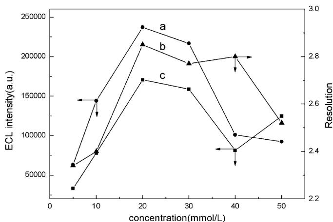
Fig. 5. Effect of running buffer concentration on ECL intensity and resolution: (a) ECL intensity of 10  $\mu\text{M}$  heroin, (b) resolution between heroin and cocaine, (c) ECL intensity of 10  $\mu\text{M}$  cocaine. Conditions: detection potential, 1.2 V; running buffer, phosphate–acetate (pH 7.2); 5 mM  $\text{Ru}(\text{bpy})_3^{2+}$  with 50 mM phosphate–acetate buffer (pH 7.2) in the detection reservoir; electrokinetic injection, 6 s at 17 kV; separation voltage, 10 kV.
