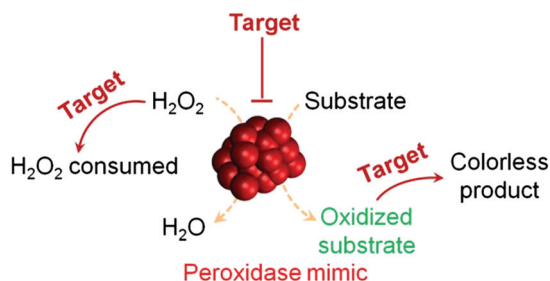
Fig. 6 By modulating the peroxidase mimics catalyzed reactions (e.g., inhibiting the nanozymes' activity, consuming H_2O_2 , or converting the coloured oxidized substrate to colourless product), the targets of interests can be detected.
